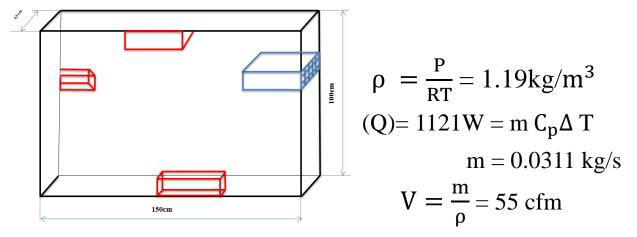
Hence fan capacity required is less when the enclosure is placed at a higher altitude than when it is placed at enclosure.
