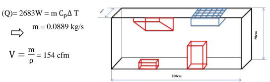
Hence the fan of capacity 154 cfm is required to maintain a operating temperature inside the enclosure with unknown humidity
